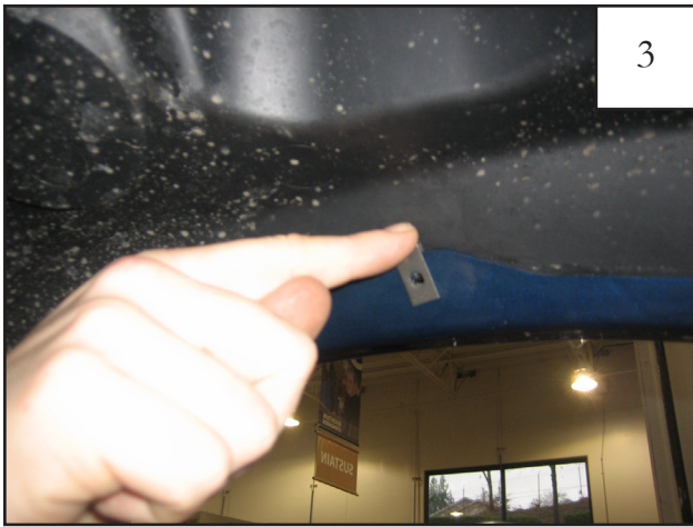
Place supplied clip (CL1-0011) over existing factory hole.
